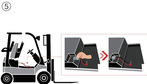
Plug in the EP Li-ion battery.
