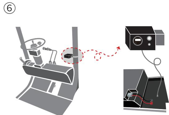
Attach the battery indicator to the cabin.
