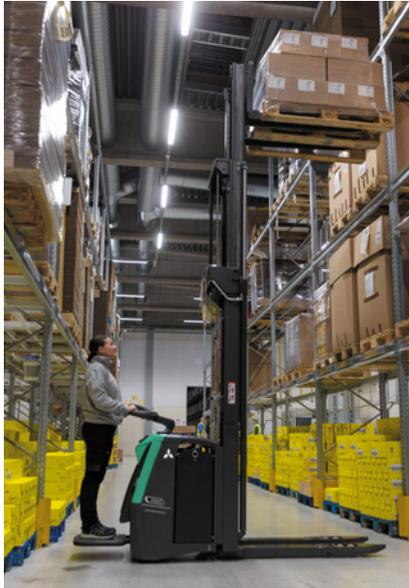
The series is available in foldable platform models with optional sidebars for use in narrow spaces, fixed platform rear entry models for fast operations where maximum operator protection is required, and fixed platform side entry models for easy on-off access on both sides for picking applications.
