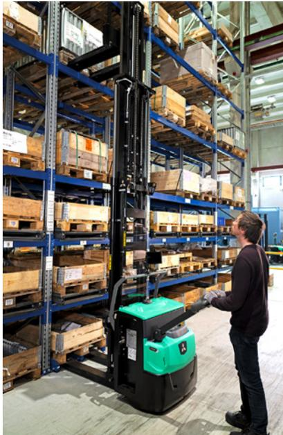
**Unaffected by dirt, debris, dust and water thanks to its sealed protective chassis and waterproof components (rated to IP54), AXiA ES will work dependably indoors or out with minimum maintenance.**
