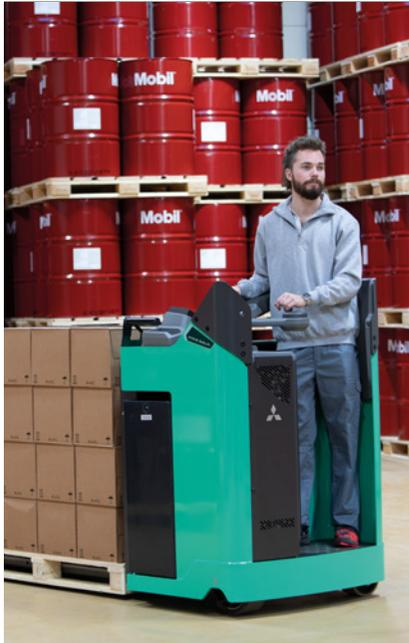
The stand-in power pallet design contains the operator completely within the truck, keeping them protected by the chassis. The stand-in concept also allows for a highly compact footprint. Along with the incredibly tight turning circle, this makes narrower aisle layouts much more feasible.
