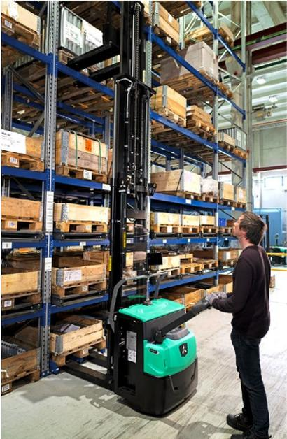
**Unaffected by dirt, debris, dust and water thanks to its sealed protective chassis and waterproof components (rated to IP54), AXiA ES will work dependably indoors and occasionally out with minimum maintenance.**
