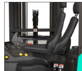
Suspension seat with tilting backrest
