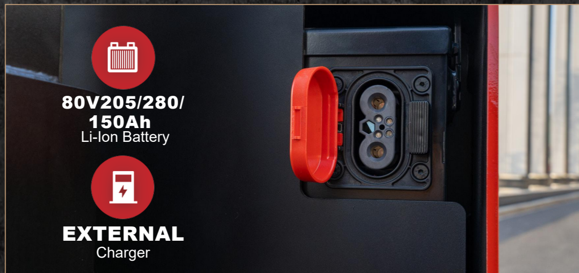
External charging port with a protective cover
